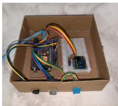
Gambar 8. Prototype Sistem Monitoring Kualitas Udara
