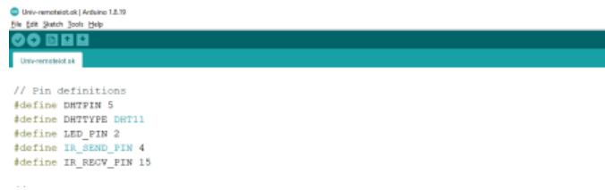
Figure 20. Pinout definition code used
