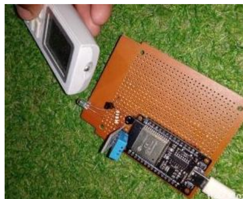
Figure 5. Recording IR code from AC Remote
