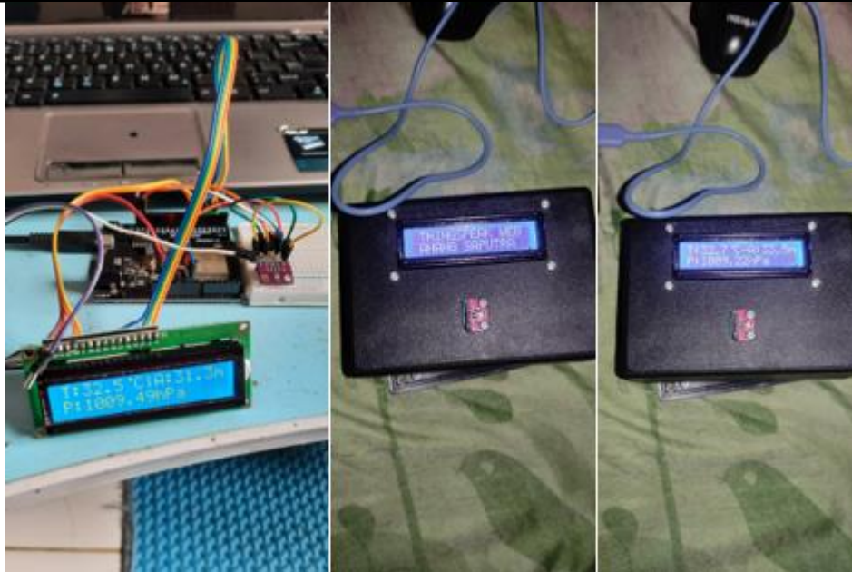
Gambar 4. Hasil Perancangan Alat Monitoring Suhu
